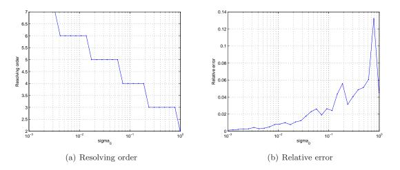
Figure 3: The resolving order  $m_0$ , for  $\sigma_0 \in [10^{-3}, 1], \tau_0 = 10^{-1}$ , and the relative error of the reconstruction within this order. As in Figure 2, we repeat the experiment 100 times and the reconstruction is taken as their mean value. The large variations of the relative error in (b) for  $\sigma_0 > 10^{-1}$  indicate the instability of the reconstruction for very noisy data.
