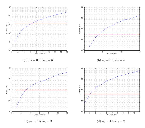
Figure 2: Relative error of the reconstructed CGPTs. For each noise level, we repeat the experiment 100 times (corresponding to 100 realizations of the noise) and the reconstruction is taken as their mean value. The horizontal solid line in each figure indicates the resolving order  $m_0$  given by (6.2) with the tolerance number  $\tau_0 = 10^{-1}$ .
