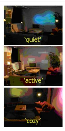
**Fig. 4** With the prototype atmosphere control system, the ambience of a room (including music, wall art projection and lights) can be changed using a personalized atmosphere model. *Left picture* a "quiet" atmosphere, created by a subtly animated blue figure on the wall. *Middle picture* an "active" atmosphere, created by bright lights, and moving blocks on the wall. *Right* a "cozy" atmosphere, created by warm colored lights, warm colored video art, and use of spotlights
