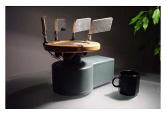
Fig. 7 With the Carrousel, a tangible interaction device, users can "sculpt" atmospheres. The stage rotation speed and the orientation of the flags can be changed to express a desired atmosphere
