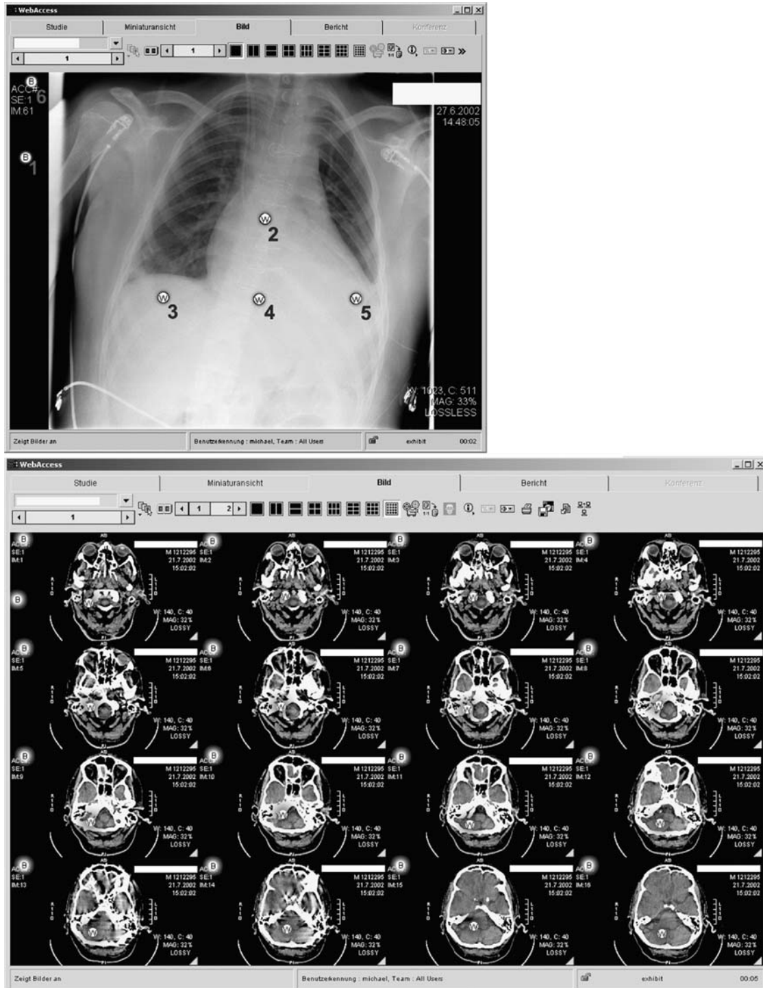
Fig 1. (a) CR images were displayed in a 1 \times 1 setting. Locations of screen pixels monitored by using method 3 are indicated by dots. The target RGB value assigned to the dots marked B was "black" and to the ones marked W "brighter than dark gray." (b) For CT and MR, always 16 images were displayed in a 4 \times 4 setting. The locations of screen pixels monitored by using method 3 are indicated by dots. The target RGB value assigned to the dots marked B was "black" and to the ones marked W "brighter than dark gray."
