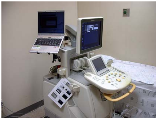
Fig 4. Portable ultrasound machine equipped with PACS device. The PACS device program is installed in a laptop computer fixed in portable ultrasound machine.
