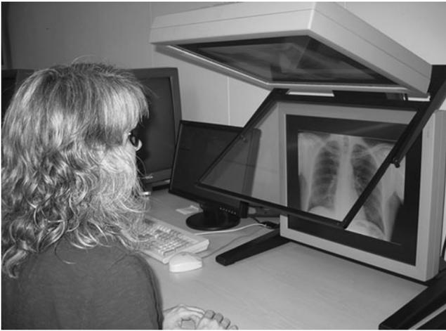
**Fig. 4** Stereographic viewing system
