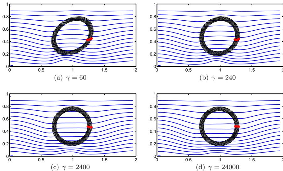
**Fig. 8** Streamlines and structure location at time  $t = 1$  for a range of stiffnesses. The red markers on the structure are used to highlight rotation and internal deformation. At the beginning of the simulation the red markers were aligned horizontally in the  $x$ -direction.
