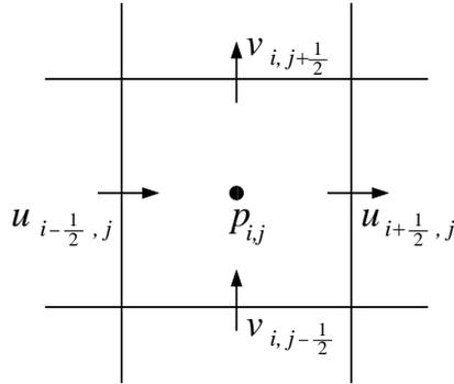
**Fig. 2** Staggered grid discretization in which the velocity field  $\mathbf{u} = (u, v)$  and Eulerian body force  $\mathbf{f} = (f_1, f_2)$  are approximated at the centers of the cell edges, and in which the pressure  $p$  is approximated at the cell centers.
