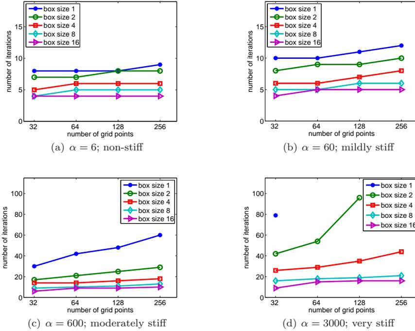
**Fig. 7** Iteration counts of MG-GMRES for different stiffnesses, box sizes, and different grid resolutions. The number of grid points refers to the number of grid cells in each direction on the Eulerian grid.
