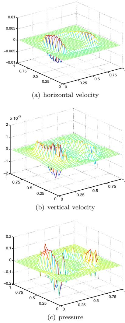
**Fig. 5** Plots of the velocity and pressure corresponding to an eigenvector of the multigrid iteration matrix with eigenvalue 0.8522 for relative stiffness  $\alpha_{\text{exp}}/\alpha$ .
