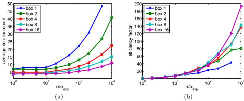
**Fig. 9** (a) Average number of iterations of the MG-GMRES method per time step in the implicit-time simulation. (b) The efficiency factor is the expected speed-up gained by using the implicit method in place of an explicit method.
