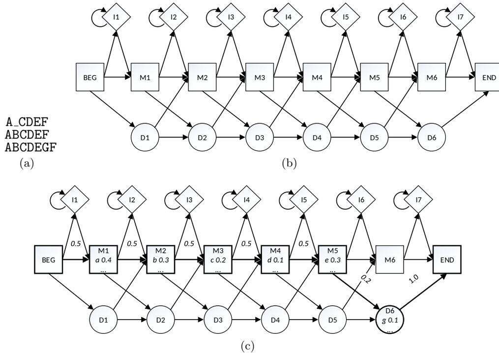
Fig. 12: Sequence set of symbols (a) are aligned using HMM (b)(c) which is a trained state machine consists of node types:  $Mx$  represents matches in index  $x$ ,  $Dx$  represents deletions in index  $x$ ,  $Ix$  represents insertions in index  $x$ , and arrows represent transitions among them.
