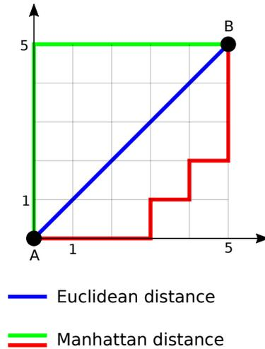
Fig. 3: Example of Euclidean and Manhattan distances between two points A and B. The Euclidean distance is  $\sqrt{5^2 + 5^2} = 7.07$  tile's length while Manhattan distance is  $5 + 5 = 10$  tile's length.
