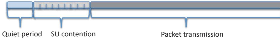
Figure 3: The structure of a time slot when CS is enabled.
