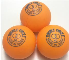
**Fig. 5** Setup for measuring the friction coefficient  $\mu$ . Three balls are arranged together in the shape of a triangle frame and placed on a flat table.
