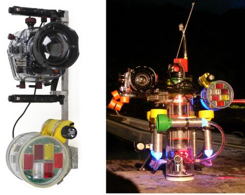
Fig. 7. (Left) The adaptive illumination device consists of six colored flashes with adjustable power. The device is attached to a standard digital camera in an underwater housing. (Right) Imaging apparatus attached to an underwater robot at the end of a mission.
