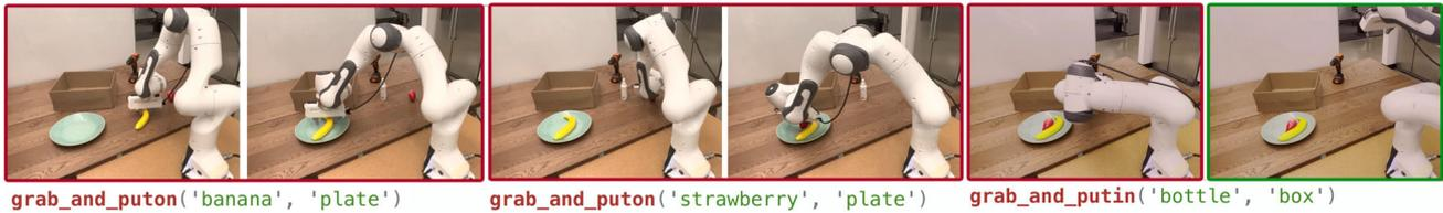
**Fig. 4** Robot plan execution rollout example on the sorting task showing relevant objects *banana*, *strawberry*, *bottle*, *plate* and *box*, and a distractor object *drill*. The LLM recognizes that *banana* and *straw-*
