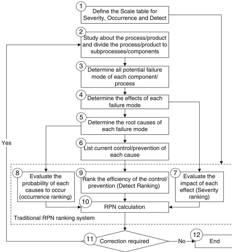
Fig. 1 The operation of FMEA
