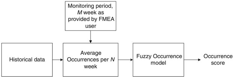
**Fig. 3** The proposed frameworks for predicting and updating the occurrence score
