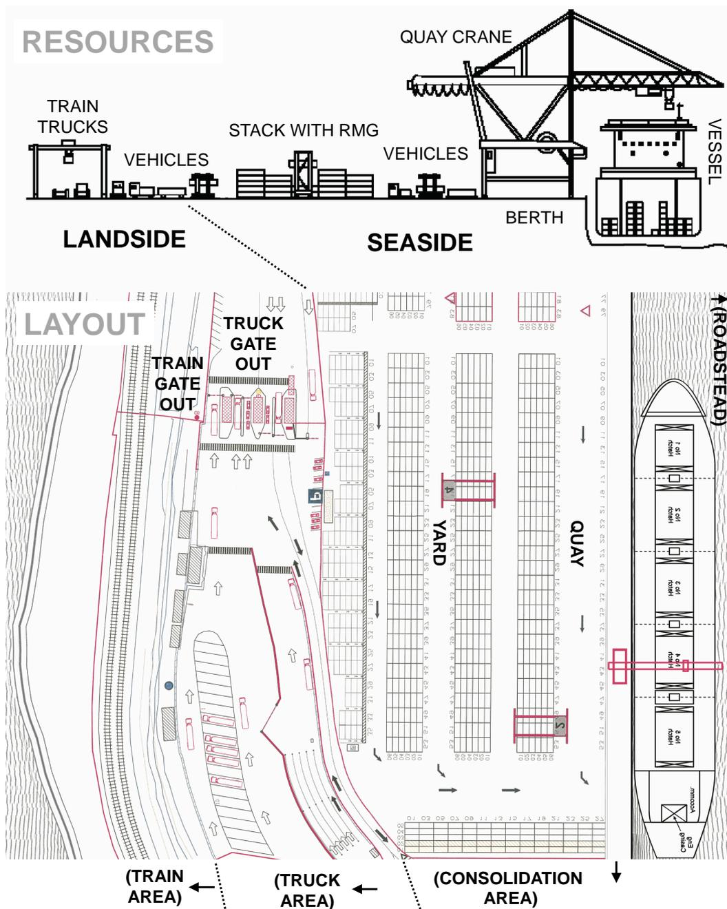
Fig. 2: Resources and layout of the pilot container terminal system
