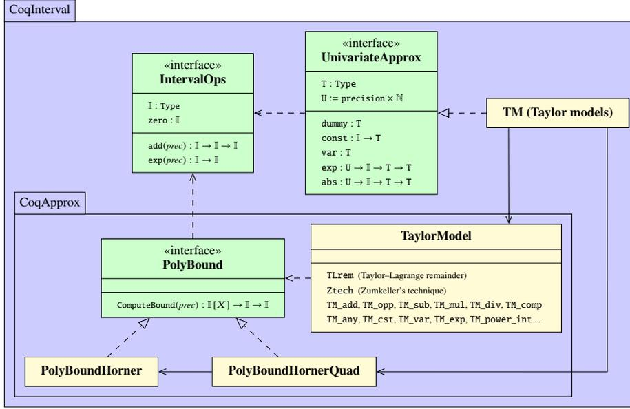
**Fig. 3** Diagram (UML) that summarizes the architecture of the CoqApprox package w.r.t. CoqInterval.
