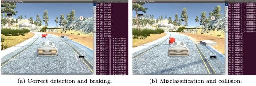
Fig. 9: Unity-Udacity simulator AEBS. The onboard camera sends images to the CNN. When a cow is detected a braking action is triggered until the car comes to a complete stop. Full videos available at <https://www.youtube.com/watch?v=Sa4oLGcHAhY> and <https://www.youtube.com/watch?v=MaRoU50gimE>.
