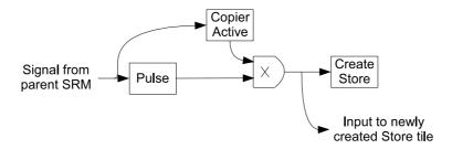
Fig. 8. The logical structure of the copier.
