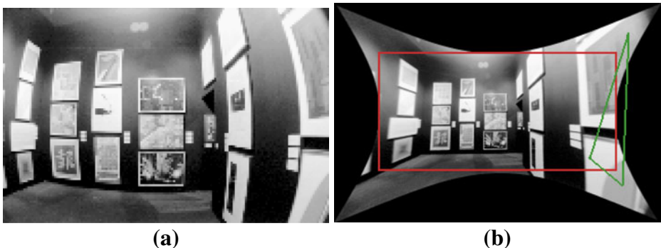
Fig. 7 a Distorted image taken by a wide angle of view lens. b Undistorted counterpart. The values in the black areas are not defined. We only store the part in the red square in the keyframe as the texture triangle in green would cause issues in the back projection to the mesh. (Courtesy of Becker)
