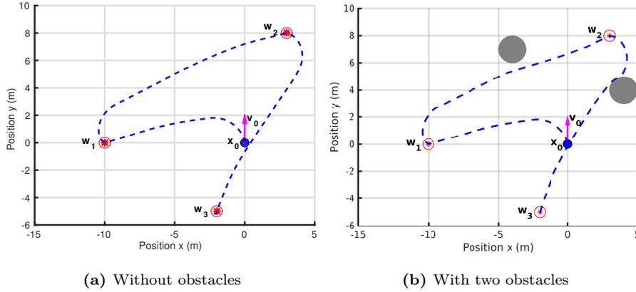
**Fig. 6** Computed paths using the path-planning algorithm
