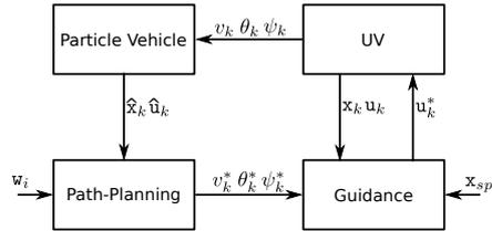
**Fig. 1** Scheme of the path-planning & guidance system
