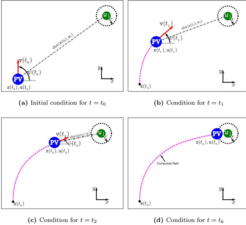
**Fig. 3** Computing a path between  $\mathbf{x}(t_0)$  and  $\mathbf{w}_1$
