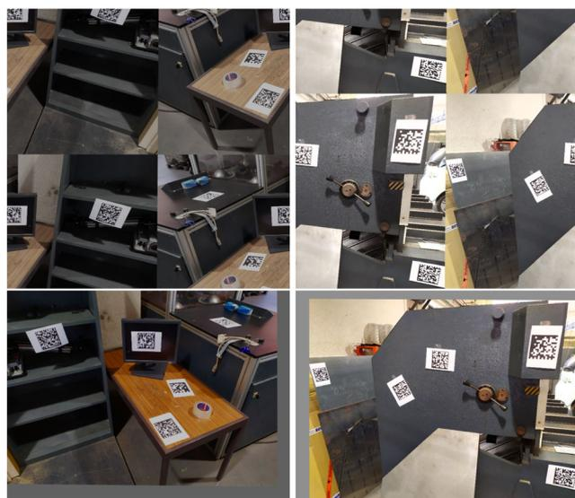
**Fig. 3** Two different data augmentation methods applied during YOLO networks training: two examples of mosaic augmented images (upper images) and random affine transformed frames at the bottom
