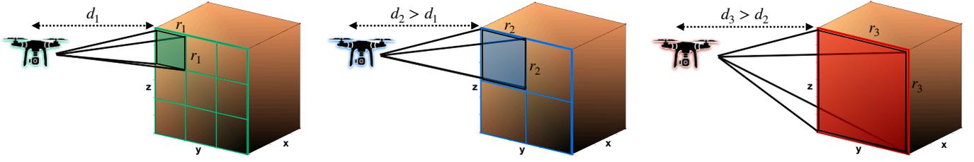
Fig. 4. The figure illustrates the projected FoV shape (i.e.,  $r_i \times r_i$  square) as a function of the distance (i.e.,  $d_i$ ) between the UAV agent and the object of interest. Assuming the distance  $d_i$  is kept constant, the UAV agent must scan each cell of the shown grid in order to search the total area of the face.
