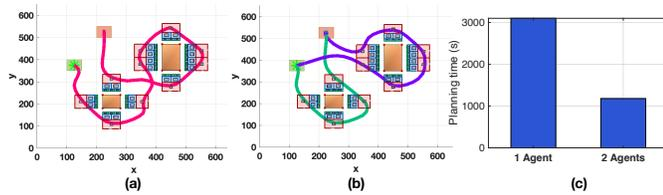
Fig. 12. The figure illustrates the decomposition of the search planning problem into smaller sub-problems. Specifically, in this scenario 2 UAV agents are used to search 2 objects of interest (each agent is assigned to a different object). (a) The search planning conducted by 1 agent, (b) the search planning conducted by 2 agents, (c) the planning time for each scenario.
