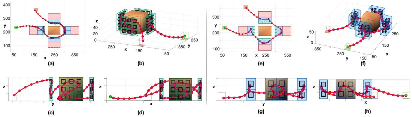
Fig. 8. The figure illustrates the generated search plan for: (a)-(d)  $Q = 0.9$  and (e)-(h)  $Q = 0.7$ . The agent passes through the appropriate zones and visits all the cuboids (and interior cubes) in its way in order to search each face of the object of interest with the desired detection probability.
