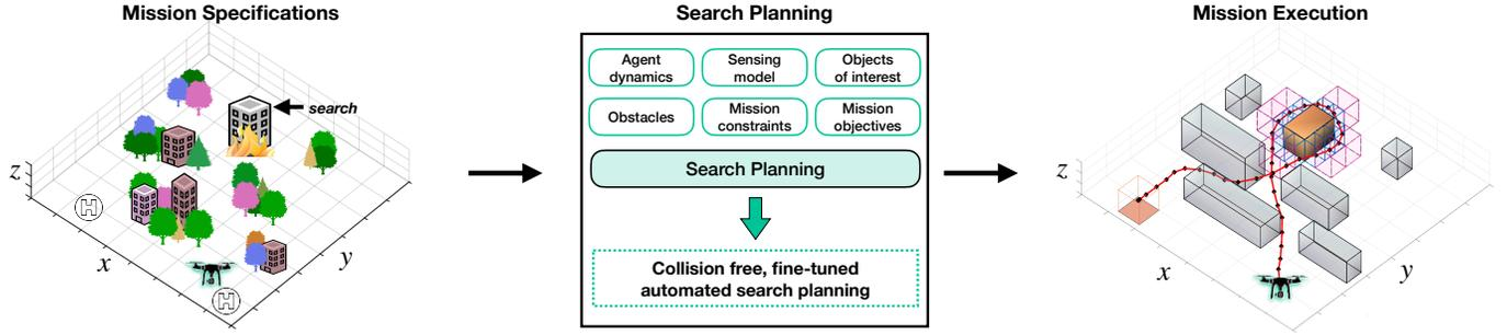
Fig. 2. Overview of the proposed search-planning framework. The proposed framework aims to automate the second and most critical phase (i.e., the search phase) of a traditional SAR mission with a single UAV agent.
