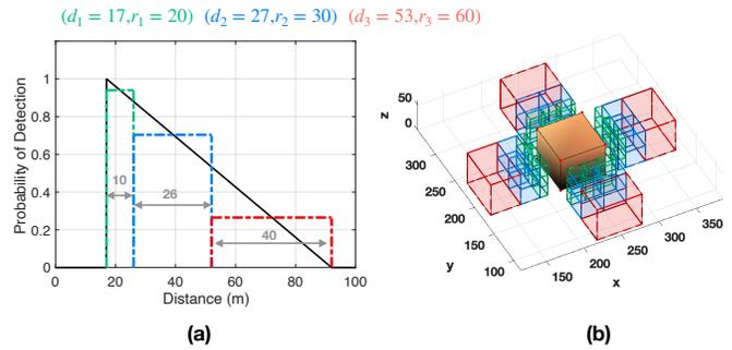
Fig. 7. The figure illustrates the 3D Zone construction step used in our experiments. a) The probability of detection has been discretized into 3 zones, b) The area discretization around the object of interest and the formation of 3 zones (i.e., green, blue and red).
