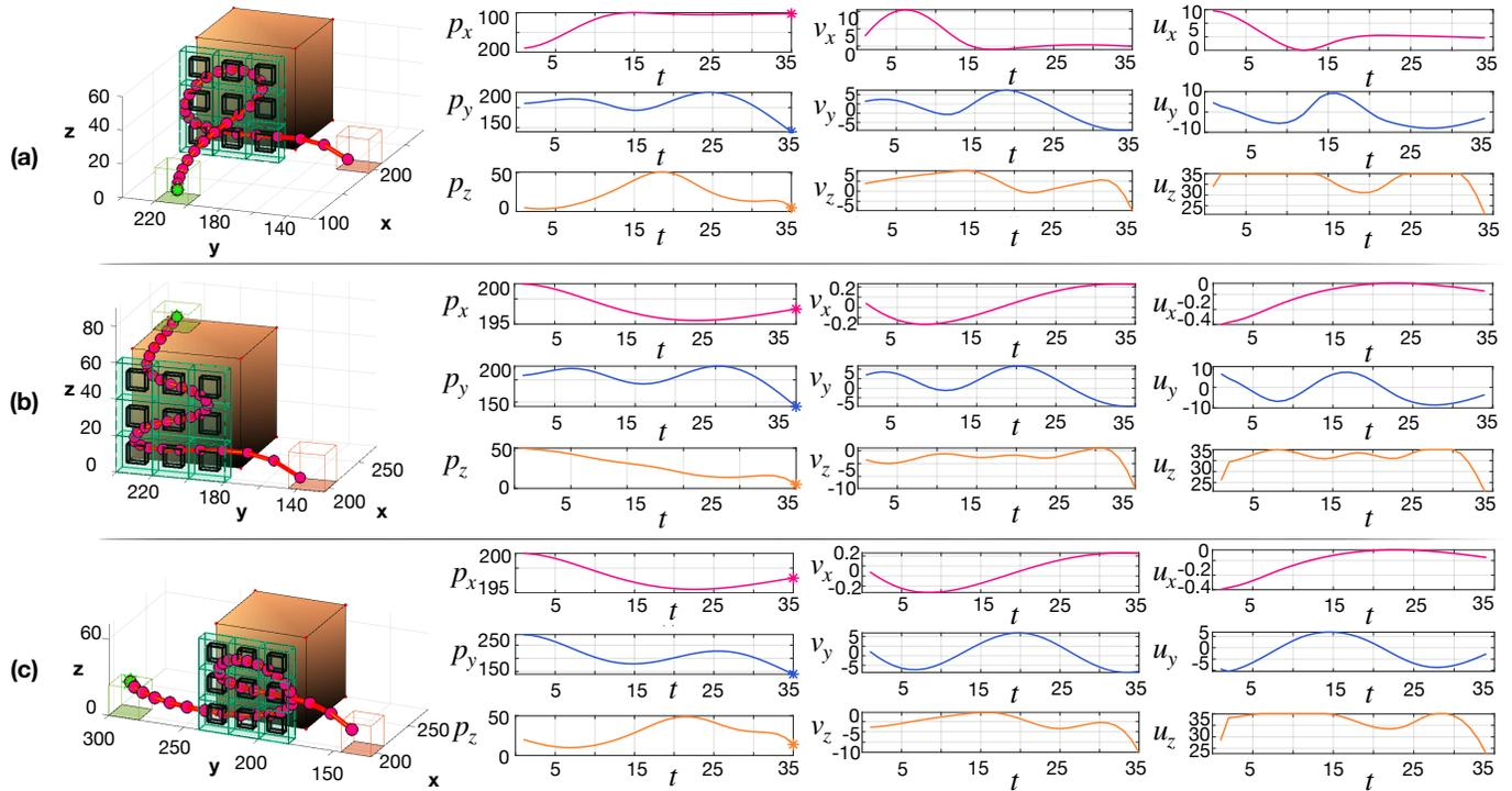
Fig. 10. The figure illustrates the various search plans generated by the proposed framework for searching a single face of an object of interest. As it is shown, depending on the agent starting position the shape of generated trajectory changes in order to optimize the mission objective while incorporating the agent dynamics.
