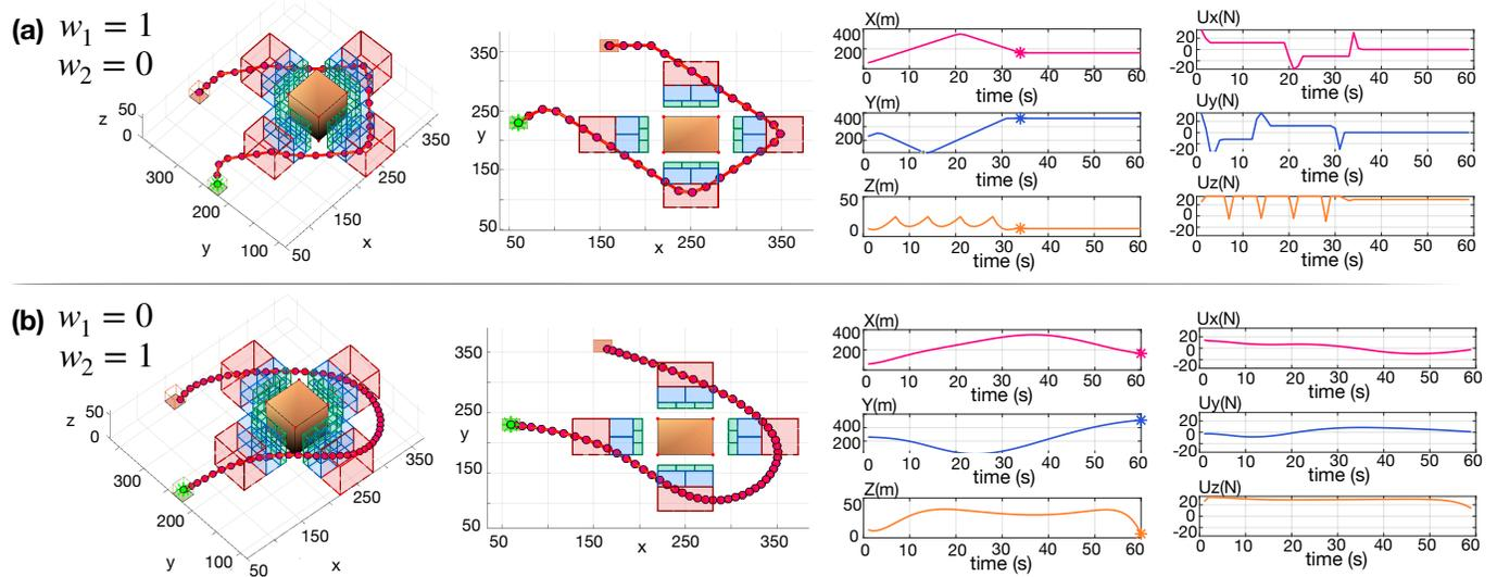
Fig. 9. The figure illustrates the effect of the weights  $w_1$  and  $w_2$  of Eqn. (11) on the generated search plan. (a) The generated search plan minimizes the mission execution time. (b) The generated plan optimizes the UAV energy efficiency by minimizing the deviations between consecutive control inputs.
