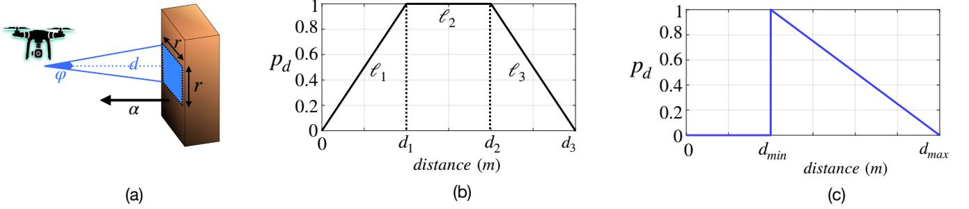
Fig. 3. The figure illustrates the agent sensing model discussed in Sec. IV-B. a) the geometry of the UAV onboard camera FoV according to Eqn. (3), b) an intuitive representation of the probability of detection  $p_d(d)$  as a function of the distance between the agent and the face to be searched, c) the probability of detection model used in this work.
