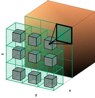
Fig. 6. The figure illustrates the interior cubes (gray) centered inside the cuboids (green). By passing through each cube the UAV agent makes sure that the whole area of the face is searched i.e., the projected FoV from within a cube encloses the area of the corresponding grid cell on the face's surface as shown in the figure.
