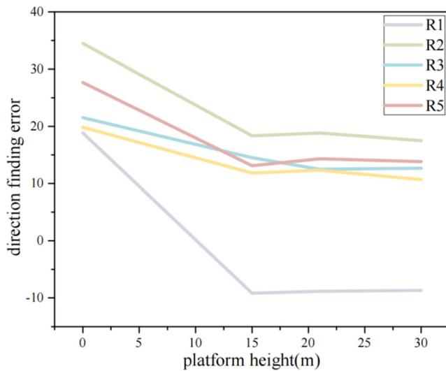
Fig. 8 The relationship between UAV platform height and direction-finding error
