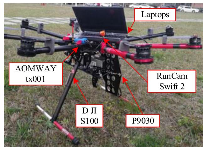
**Fig. 3** Physical image of RFI aerial monitoring system
