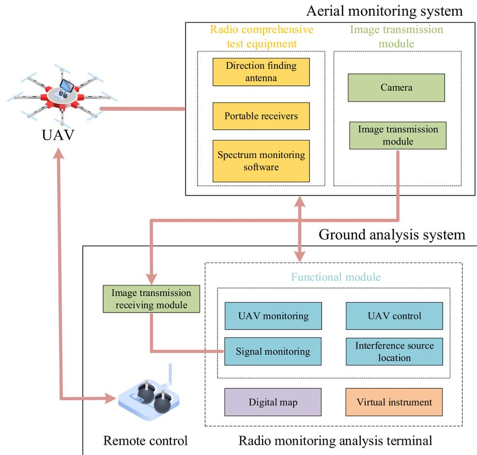
real time, therefore, a set of an image transmission device is needed to transmit the over-the-air monitoring screen to the ground terminal. In this study, the image transmission module includes a camera RunCam Swift 2, and an image transmitter module AOMWAY tx001. The camera is used to capture the spectrogram of the radio signal displayed in real time by the laptop. The image transmitter module is used to transmit the spectrum monitoring images to the ground immediately.
