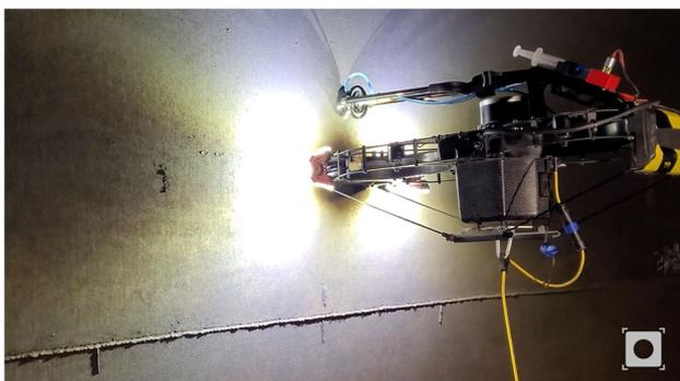
**Fig. 4** A ScoutDI prototype drone during an ultrasound inspection of a storage tank. Courtesy ScoutDI
