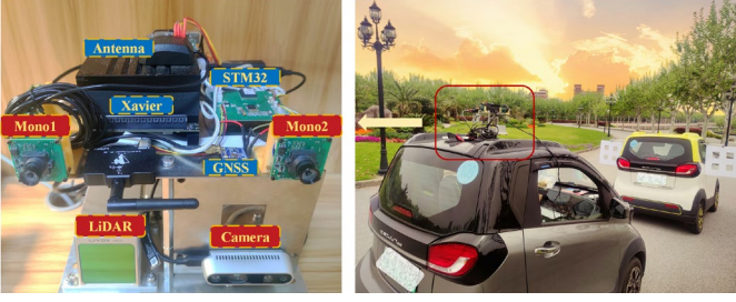
Figure 6. Multi-sensor suite and road test. Two calibration boards are placed in the front vehicle, and the suite is attached to the following car via suckers to collect data.
