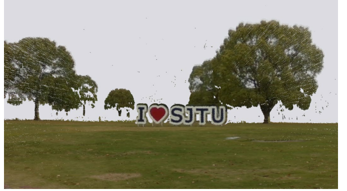
Figure 1. Colorized point cloud visualization using the estimated extrinsic parameters from our approach. The uncolored point cloud lacks pixel information, owing to the devices relative position and field-of-view (FoV).
