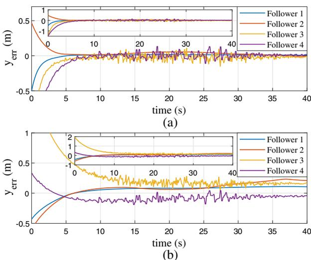
**Fig. 11** Position tracking errors on the y-axis. (a) Using ANFTSMC. (b) Using ISMC
