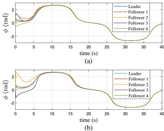
**Fig. 7** Consensus of orientations. (a) Using ANFTSMC. (b) Using ISMC
