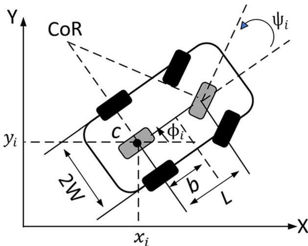
Fig. 1 Car-like vehicle reference frame and parameters
