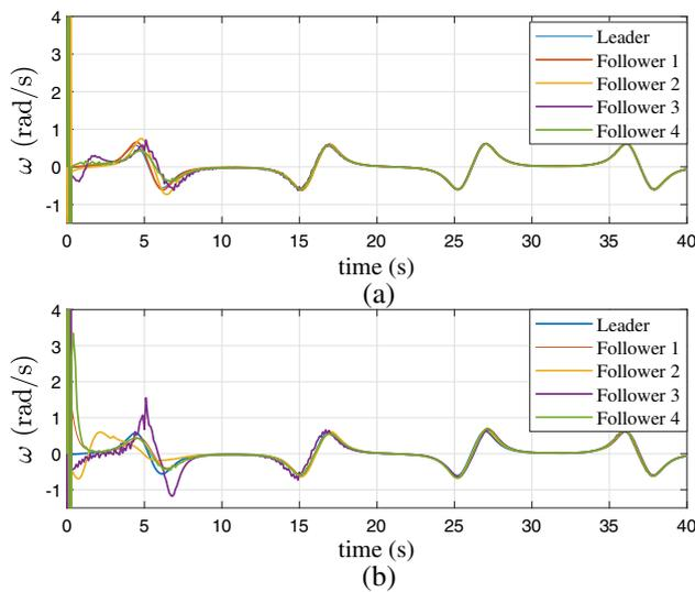
**Fig. 6** Consensus of steering velocity. (a) Using ANFTSMC. (b) Using ISMC
