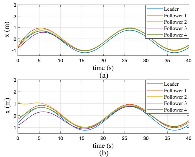
**Fig. 8** Consensus of positions. (a) Trajectories tracking on the x-axis using ANFTSMC. (b) Trajectories tracking on the x-axis using ISMC
