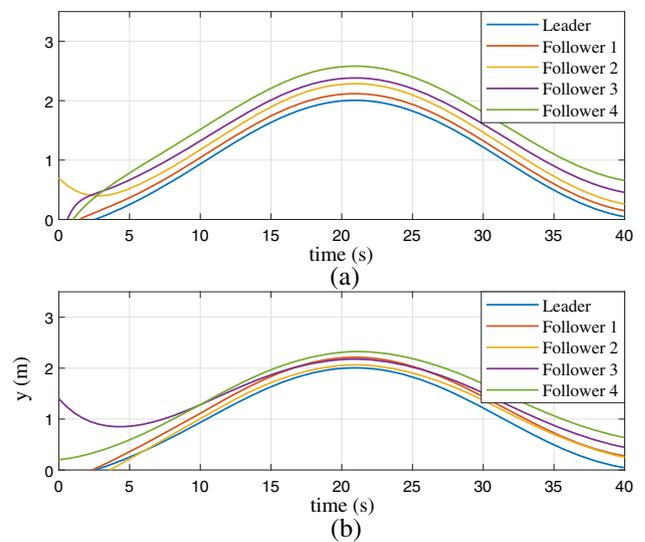
**Fig. 9** Consensus of positions. (a) Trajectories tracking on the y-axis using ANFTSMC. (b) Trajectories tracking on the y-axis using ISMC
