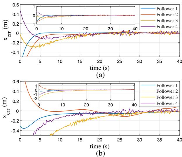
**Fig. 10** Position tracking errors on the x-axis. (a) Using ANFTSMC. (b) Using ISMC
