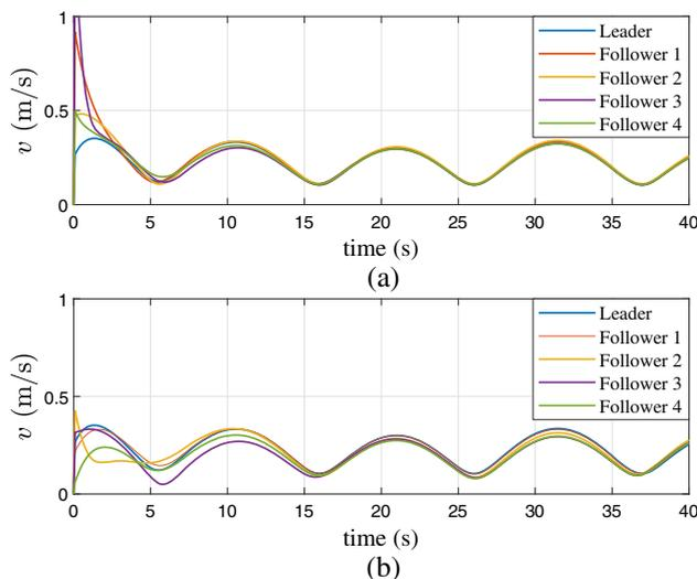
**Fig. 5** Consensus of linear velocities. (a) Using ANFTSMC. (b) Using ISMC
