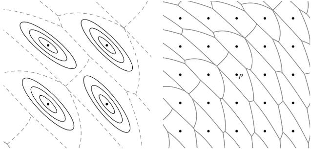
Figure 2: The distance  $\delta_p(q)$ , from a grid point  $p$  to  $q \in \mathbb{R}^2$ , is defined in terms of the local metric  $\mathbf{M}(p)$ , see (14). The level lines  $\{q \in \mathbb{R}^2; \delta_p(q) = r\}$  are ellipses (left). The collection of points  $q \in \mathbb{R}^2$  closer to  $p$  than to any other grid point is the Voronoi region of  $p$  (left: the boundaries of Voronoi regions are shown dashed). The Voronoi diagram (right) is the collection of all Voronoi regions.
