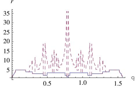
Figure 7: Radius of the AD-LBR stencil (plain), and of the A-NN stencil (dashed), for a matrix  $D_\theta$  of anisotropy ratio  $\kappa = 10$  and eigenvector  $(\cos \theta, \sin \theta)$ . The AD-LBR stencil is here always the smallest, and its radius does not exceed 5.1, versus 36.1 for A-NN.
