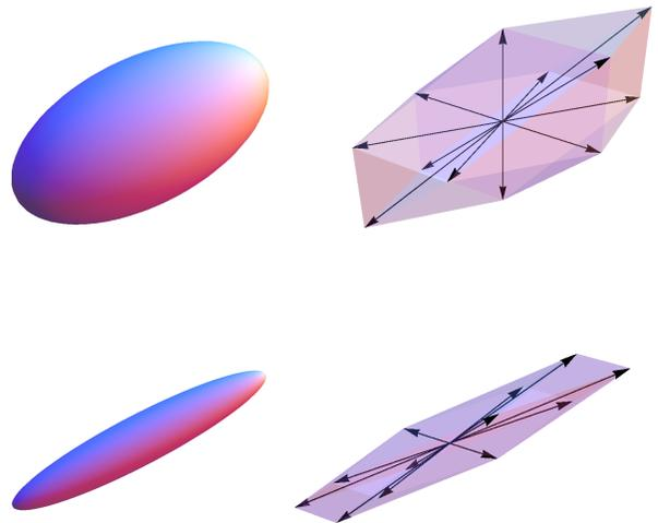
Figure 4: Right: stencil of the AD-LBR, for a symmetric matrix of eigenvector  $M$  of anisotropy ratio  $\kappa(M)$  equal to 2 (top) or 6 (bottom). The anisotropy is of “needle” type: the two largest eigenvalues of  $M$  are equal, and the needle orientation is given by the vector  $(4, 2, 3)$ . The ellipsoid  $\{z \in \mathbb{R}^3; \|z\| \leq 1\}$  is shown left.
