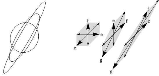
Figure 1: Right: the stencils associated to three matrices  $M$  of anisotropy ratios  $\kappa(M)$  equal to 1.1, 3.5, 8 respectively. The ellipses  $\{z \in \mathbb{R}^2; \|z\|_M = 1\}$  are shown left; their principal axis is aligned with  $(\cos(\pi/3), \sin(\pi/3))$ . More stencils are shown in [14].
