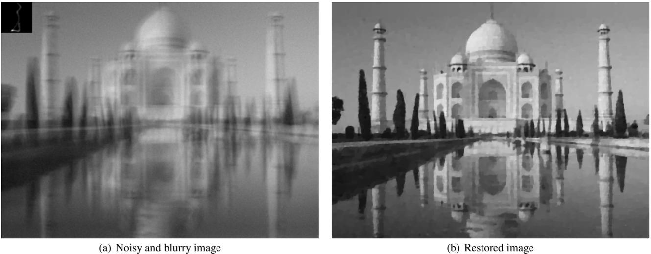
Fig. 6 Application to total variation based image deconvolution with  $\ell_2$  fitting term. (a) shows the noisy ( $\sigma = 0.01$ ) and blurry input image together with the known point spread function, and (b) shows the restored image using  $\lambda = 1000$ .
