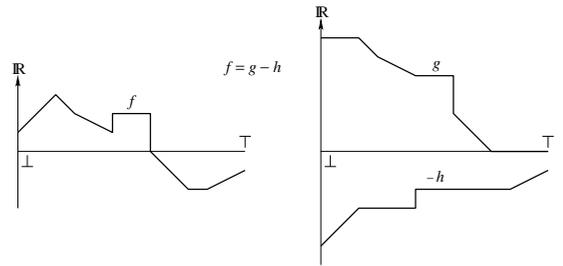
**Fig. 1** Let  $P = [\perp, \top] \subset \mathbb{R}$ . Left: a  $BV$  function  $f : P \rightarrow \mathbb{R}$ . We have  $f = g - h$  for  $g = f_P^*$  and  $h = f_N^*$ , cf. (12). Right: we show  $g$  and  $-h$ . When  $f$  decreases,  $g$  decreases while  $h$  remains constant; when  $f$  increases,  $-h$  increases (so  $h$  decreases) while  $g$  remains constant.
