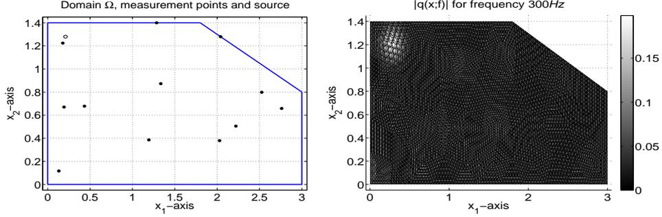
FIGURE 4.1. Acoustic domain  $\Omega$  and  $n_m = 12$  measurement points (\*) for the sound pressure and loud speaker ( $\circ$ ) (left plot); absolute value of the source function for frequency  $f = 300$  (right plot).
