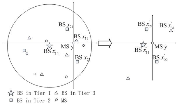
**Fig. 1** By TPNM, each tier is scaled by using the location of a specific MS  $y$  as the scaling center.
