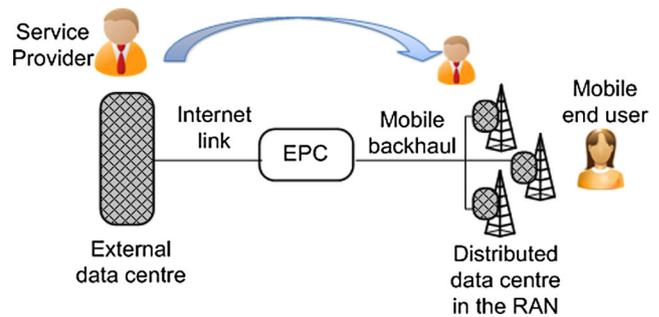
Fig. 3 System concept and impact on service deployment
