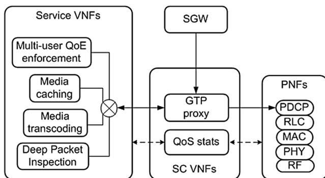
**Fig. 6** Solution for traffic forwarding at mobile edge
