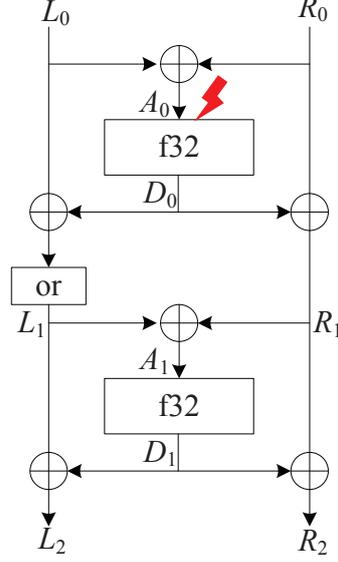
**Fig. 4.** Two round Lai-Massey scheme in a fault model
