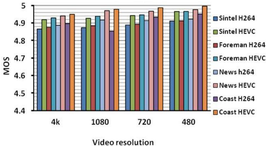
Fig. 3 Objective MOS video quality assessment for a range of resolutions and either H.264/AVC or HEVC codec, showing improved MOS for HEVC when there are no packet losses. Notice the truncated vertical scale.
