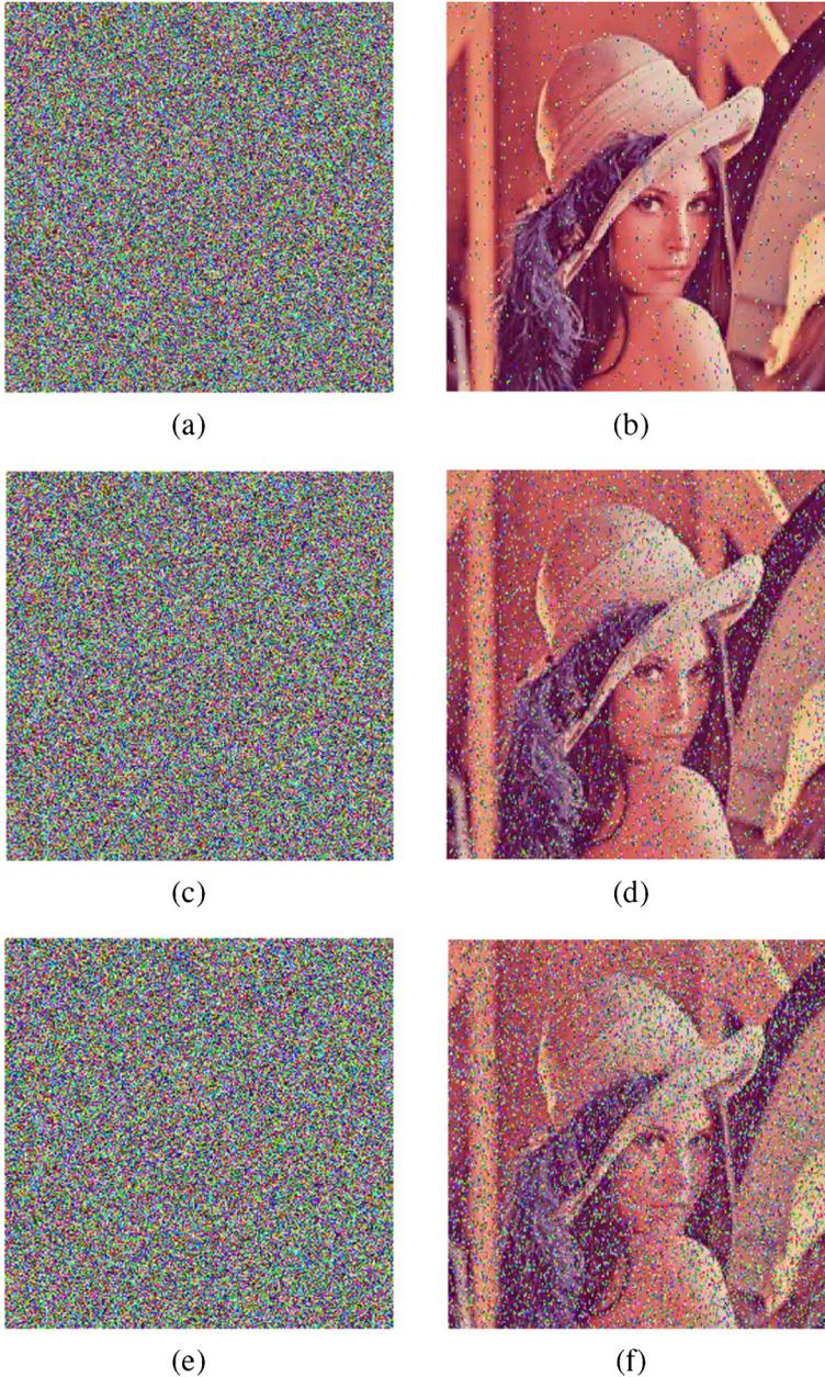
**Fig. 13** Experimental results for the performance evaluation of data loss attacks: (a, c, e) cipher images with 1%, 5% and 10% salt and pepper noise, (b, d, f) decryption results of corresponding images using our scheme
