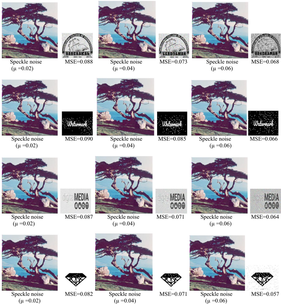
Fig. 14 Extracted watermarks “College logo”, “Watermark”, “Digital media” and “Diamond” from the attacked “Tree” images against speckle noise
