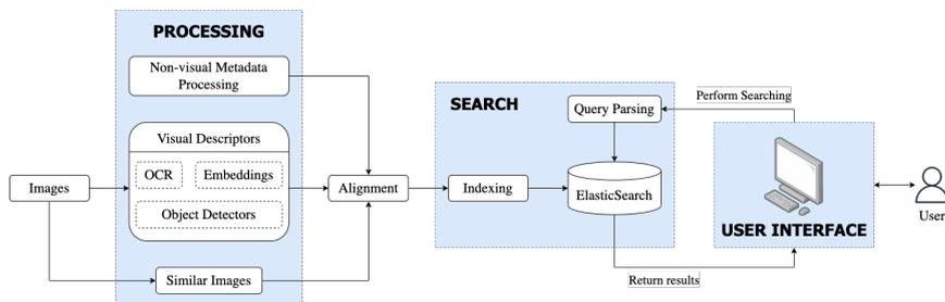
**Fig. 1** Pipeline of Myscéal which contains three main components: Processing, Search, and User Interface.
