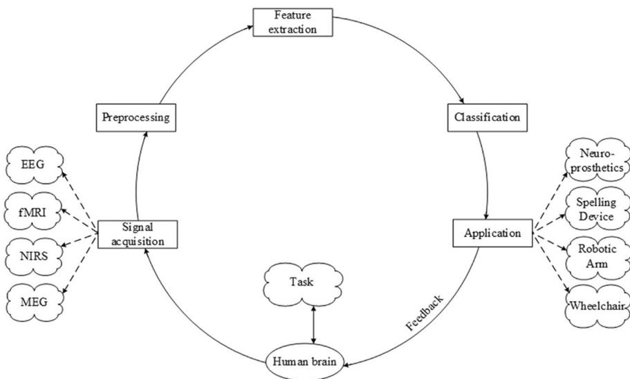
Fig. 4 Typical BCI components
