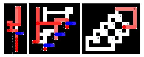
Figure 19: Custom logic can be compact. Each counter above uses the clock sequence  $\langle d, \ell, u, r \rangle$  and resets after 8 cycles (32 moves). (Left) an arrangement that cyclically counts from zero to seven: seven particles, one  $2\times1$  slider,  $8\times18$  area. (Center) a binary counter with three bits: three particles, three  $2\times1$  sliders,  $14\times14$  area. (Right) a gadget that resets every 32 moves: one particle,  $16\times14$  area.
