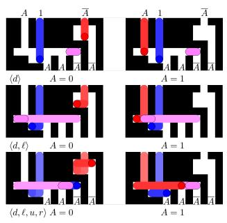
Figure 14: A single input, two-output FAN-OUT gate. This gate requires a dual-rail input, a supply particle, and a  $2 \times 1$  slider. The *clockwise* control sequence  $\langle d, \ell, u, r \rangle$  duplicates the dual-rail input.
