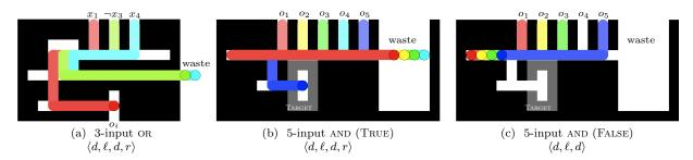
Figure 4: Gadgets that use the cycle  $\langle d, \ell, d, r \rangle$ . The 3-input or gadget outputs one particle if at least one particle enters in an input line and sends any extra particle(s) to a waste receptacle. The 5-input and gadget outputs one particle to the Target Location, marked in gray, if at least 5 inputs are True. Excess particles are sent to a waste receptacle.
