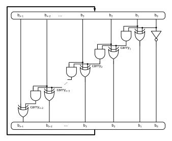
Figure 18: Gate-level diagram for an n-bit counter.
