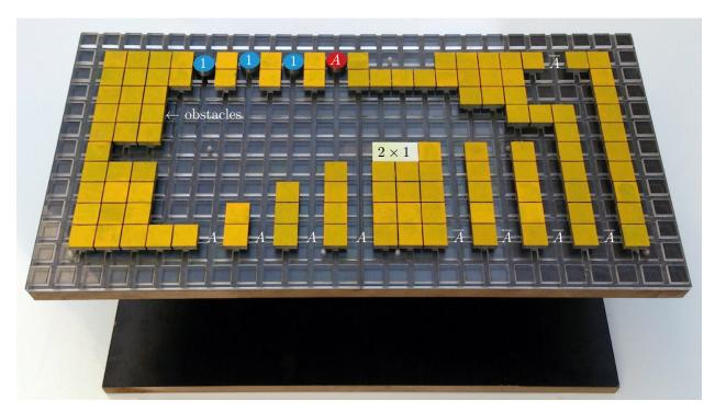
Figure 12: Gravity-fed hardware implementation of particle computation. The reconfigurable prototype is arranged using obstacle blocks (yellow) as a FAN-OUT gate using a 2×1 particle (white), three supply particles (blue), and one red dual-rail input (red). This paper proves that such a gate is impossible using only 1×1 particles. See the demonstrations in the video [9], https://youtu.be/H6o9DTIfkn0.
