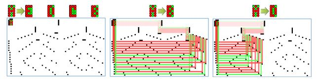
Figure 8: For any set of k fixed, but arbitrary permutations of N particles, we can construct a set of O(kN) obstacles, such that we can switch from a start arrangement into any of the k permutations using at most  $O(\log k)$  force-field moves. Here k = 4 and 'A' is transformed into 'B', C', 'D', or 'E' in eight moves:  $\langle r, d, (r/\ell), d, (r/\ell), d, \ell, u \rangle$ .
