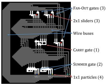
Figure 17: A three-bit counter implemented with particles. The counter requires three FAN-OUT gates, two summer gates, and one carry gate. Six  $1\times1$  particles and three  $2\times1$  particles are used. The gates and wire buses are actuated by the CW sequence  $\langle d, \ell, u, r \rangle$ . See video at https://youtu.be/QRAOaLZjuBY?t=4m9s for animation.
