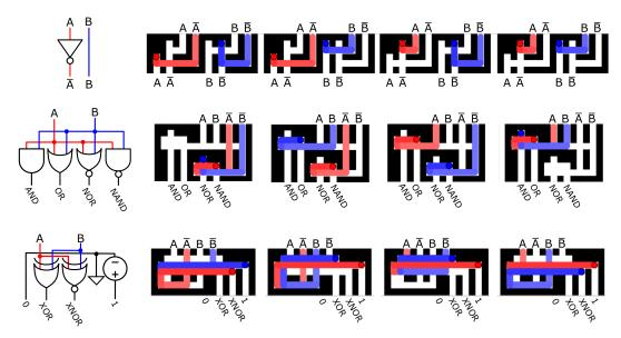
Figure 10: Schematic and diagram of dual-rail logic gates. Each gate employs the same clock sequence  $\langle d, \ell, u, r \rangle$ , the four inputs correspond to  $A, \bar{A}, B, \bar{B}$ . The top row is a NOT gate and a connector. The middle row is a universal logic gate whose four outputs are AND, NAND, OR, NOR. The bottom row gate outputs the XOR, XNOR of the inputs and constants 1 and 0. See video at http://youtu.be/mJWl-PgfosO for a hardware demonstration.
