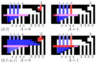
Figure 15: The FAN-OUT gate can drive multiple outputs. Here a single input drives four outputs. This gate requires a dual-rail input, three supply particles, and a  $2 \times 1$  slider. The clockwise control sequence  $\langle d, \ell, u, r \rangle$  quadruples the dual-rail input.
