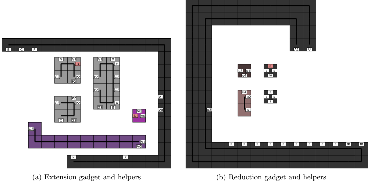
Figure 11: (a) The path extension gadget (dark grey) also has information-specific versions. The light grey assemblies attach piece-by-piece to form a path portion. The purple helpers are used to detach the extension gadget, along with the info block that allowed this extension. (b) The tape reduction gadget (dark grey) attaches once a given tape section has already been read. The reduction helpers (red and dark grey) attach to the gadget, and build up the repulsive force that is responsible for the destabilization of the gadget, along with the previously read tape section.
