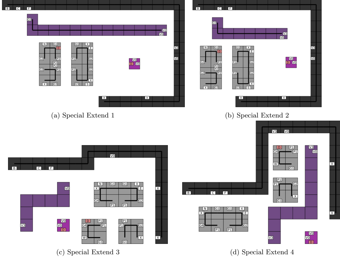
Figure 22: These are the special-case extension gadgets. While slightly different, all extension gadgets utilize the same mechanics shown in Section 4. (a-d) The B , C , F , X glues on the extension gadgets (dark grey) are used for gadget attachment. The second X glue allows the first portions of the new path piece (light grey) to attach. The V glues are utilized by the extension helpers (purple) in order to detach the gadget.
