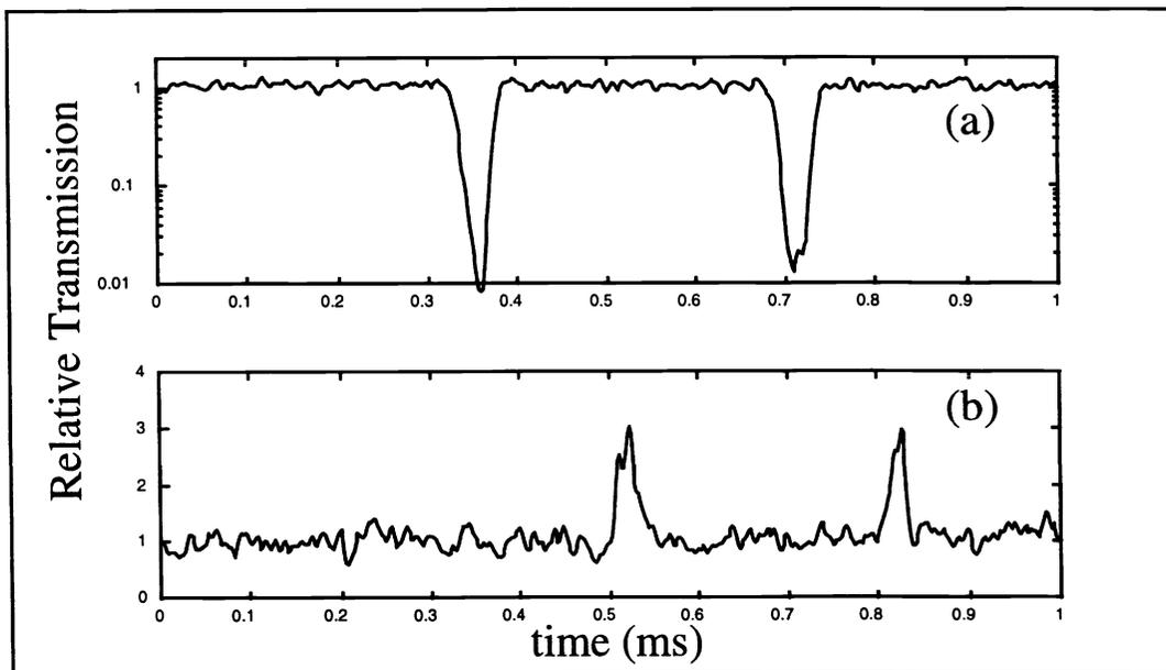
**Figure 3.** Real-time changes in transmission of the atom-cavity system produced by the transit of individual atoms through the cavity mode. In (a) the probe is tuned close to the coincident atom-cavity resonance (detuned by  $-20\text{MHz}$ ), and decreases in transmission by two orders of magnitude are observed. In (b) the probe is detuned by  $\approx -g_0 = 120\text{MHz}$ . Here atom transits give increases in transmission.
