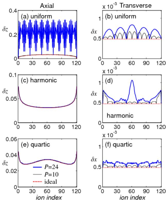
FIG. 5: (Color online) The distributions of the axial and transverse PF (in units of  $d_0$ ) under the periodic cooling for (a)(b) a uniform array, (c)(d) a harmonic trap, (e)(f) a quartic trap. The total number of ions  $N = 121$ . All parameters are the same as in Fig. 3 except for the ancilla arrangement. The curve legend for all six panels is the same and is given in (e).
