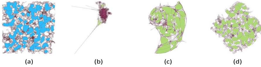
Fig. 22: Layouts of sparse WSN with n = 1,000 and d = 8 . (a) ground truth, (b) layout generated by the DH algorithm, (c) layout generated by the FA2 algorithm, and (d) layout generated by the KK-MS-DS algorithm.
