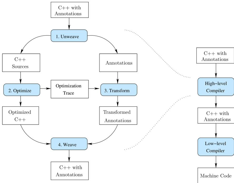
**Fig. 14** Work-flow of the source-to-source high-level compiler
