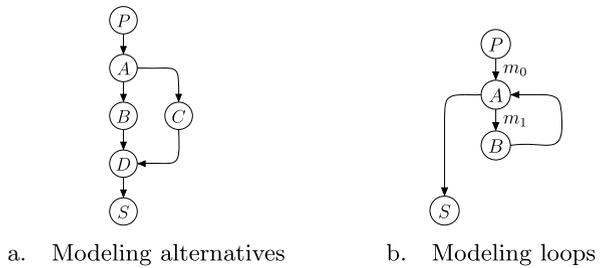
The structure of the resulting IPET constraints is explained with help of two examples, with  $P$  standing for predecessor node and  $S$  for successor node (Fig. 1).
