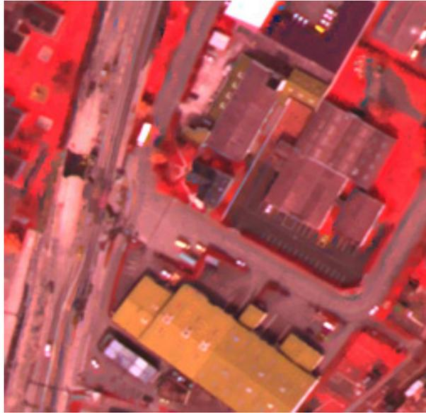
Figure 9: the  $R, G, IR$  channels of the reconstructed image (at the resolution of the panchromatic image) obtained using functional (19) with  $p = 2$ .
