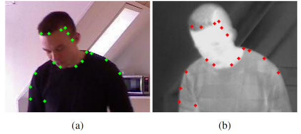
Fig. 5: Example of \text{RGB} (a) \Rightarrow \text{thermal} (b) registration.
