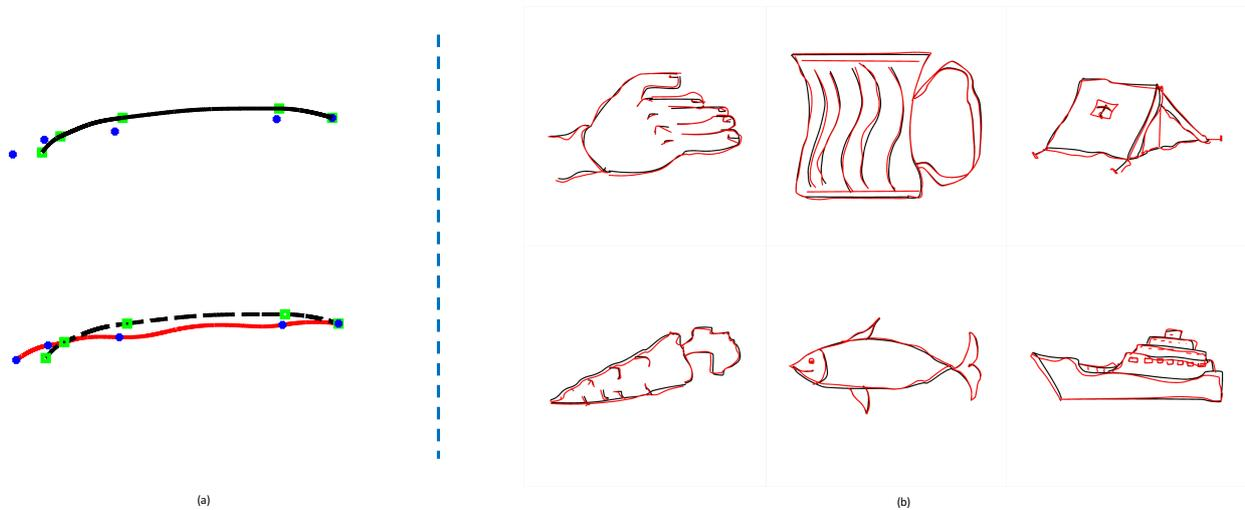
**Fig. 4** Local sketch deformation. (a) demonstrates how we do local deformation. The green squares represent control points while the blue dots are the new deformed positions of these points. (b) shows several example sketches with local deformation. The original stroke are shown in black while the distorted ones are in red.
