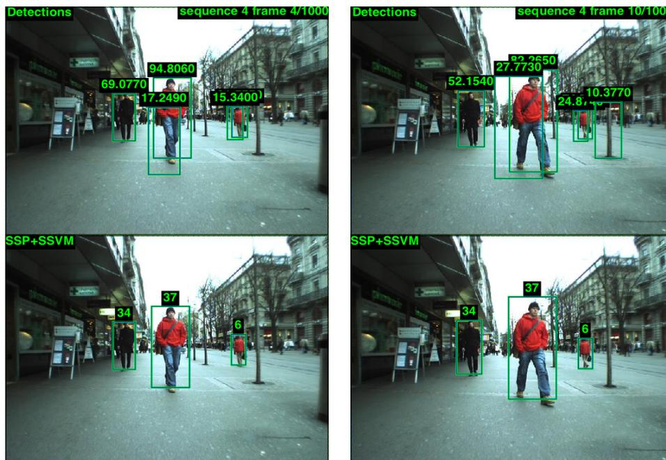
Fig. 9: By learning a proper parameter set, even a network-flow model without pairwise potentials can prune away many false tracks by reasoning about detection confidence and transition smoothness.
