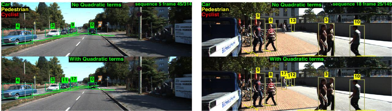
Fig. 7: Additional Qualitative Results on KITTI DPM detection set. With help of intra-class quadratic interactions, the tracker is able to instantiate more correct trajectories.
