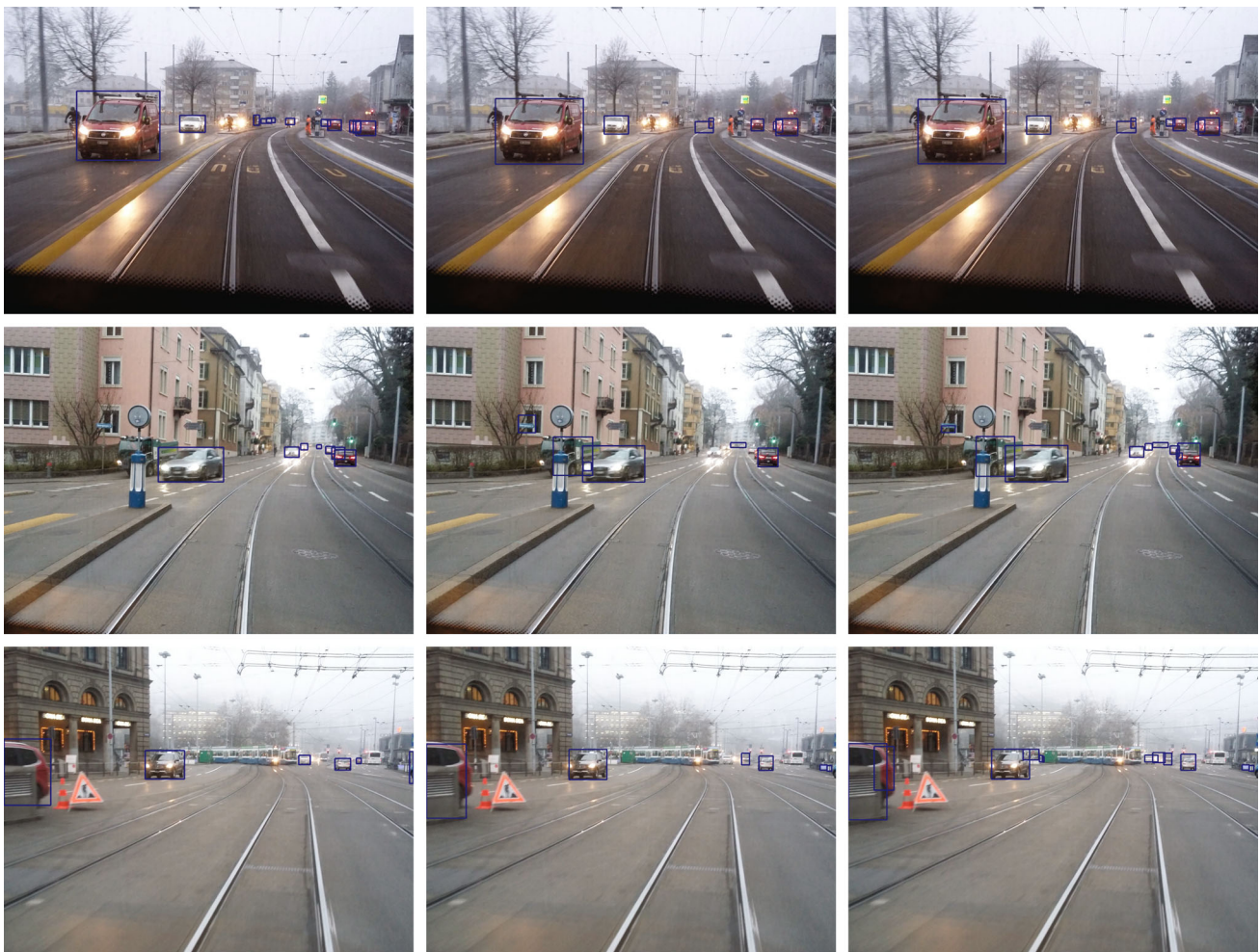
Fig. 12 Qualitative results for detection of cars on Foggy Driving . From left to right: ground truth annotation, baseline Fast R-CNN model trained on original Cityscapes, and our model FT-0.005 fine-tuned on Foggy Cityscapes-refined with light fog. This figure is seen better when zoomed in on a screen
