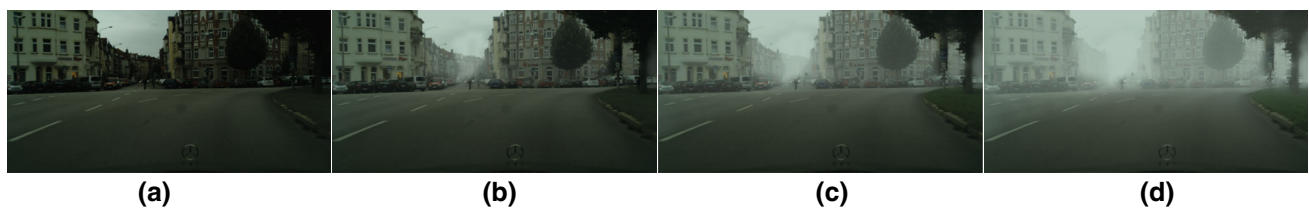
Fig. 4 Different versions of an exemplar scene from Foggy Cityscapes for varying visibility. a clear-weather. b \beta = 0.005 . c \beta = 0.01 . d \beta = 0.02
