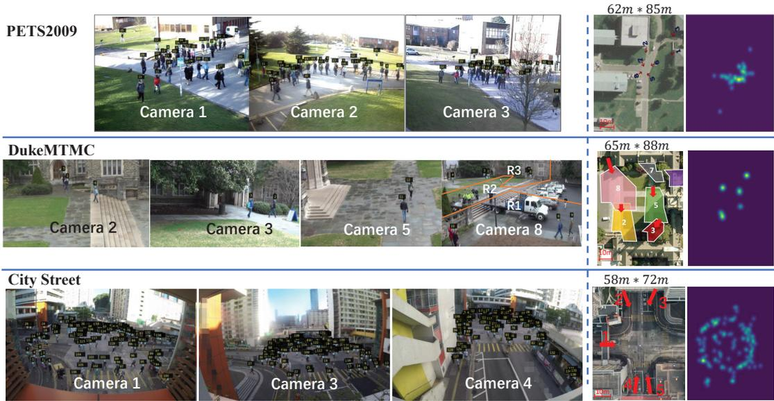
**Fig. 13** Examples from 3 multi-view counting datasets. The first column shows the camera frames and annotations. The second column shows the camera layout and scene-level ground-plane density maps. Note that ‘R2’ region of Camera 8 of DukeMTMC dataset is not used since no annotations are available.
