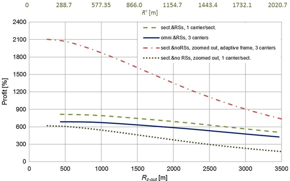
**Fig. 10** Comparison of the economic performance between omnidirectional (three carriers) and tri-sectored (one carrier/sector) BSs in the presence of relays and with the central BS coverage zone zoomed out. RSs coverages are zoomed into zero. All plots are under the same total DL BW, and  $K = 3$
