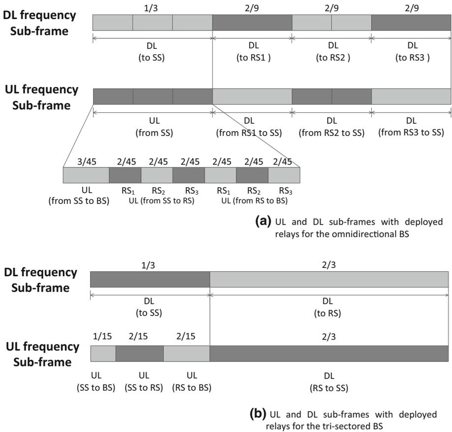
**Fig. 5** Structure for UL and DL sub-frames with deployed relays, **a** omnidirectional BS, **b** the tri-sectored BS
