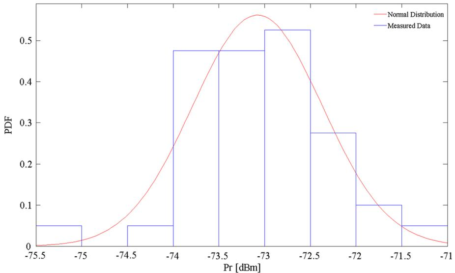
**Fig. 1** Distribution of the terminal received power (dBm) for a measurement point taken in Covilhã. The superimposed Gaussian curve (in dB) suggests that the terminal received power approximately according to a log-normal distribution
