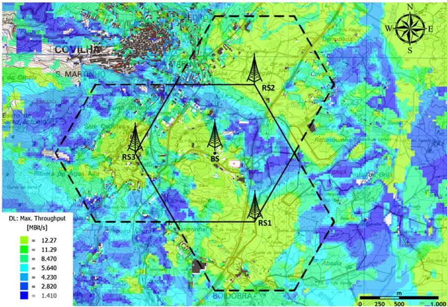
**Fig. 9** Spatial variation of the throughput with tri-sectored BS antenna and the presence of relays with RT
