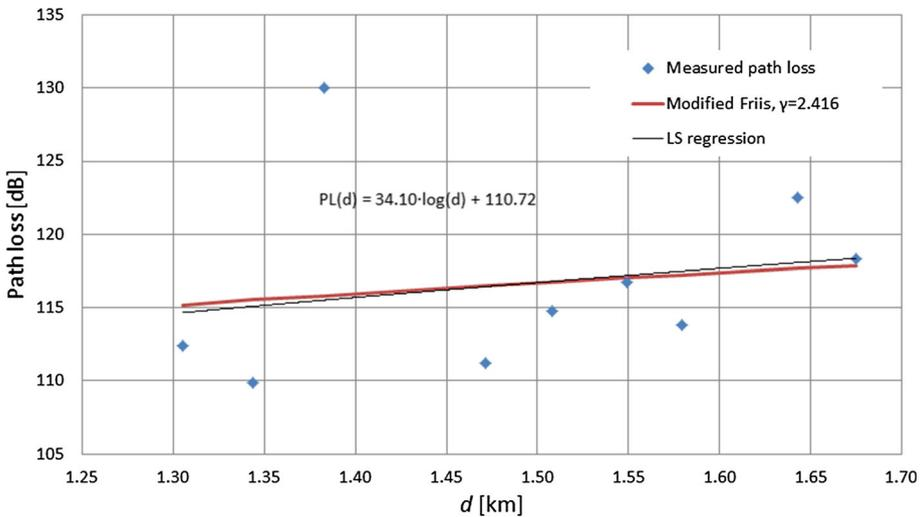
**Fig. 2** Measured and modified Friis ( $\gamma = 2.416$ ) path loss curve
