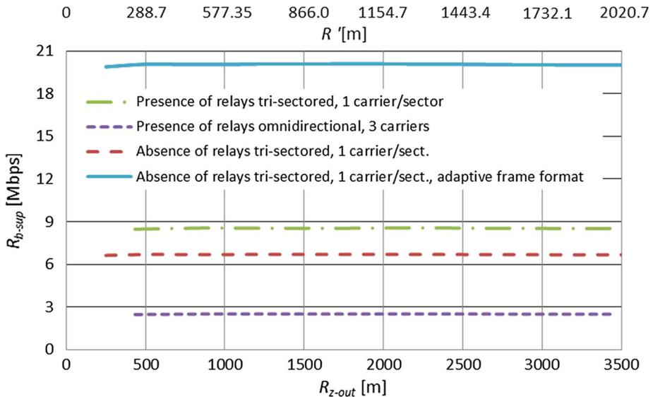
**Fig. 6** Comparison of the equivalent supported throughput between the cells with relays and the zoomed-out cells,  $K = 3$
