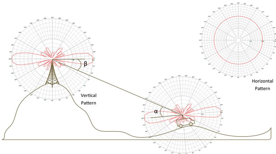
**Fig. 3** Influence of the angles of incidence and arrival in the computation of the path loss
