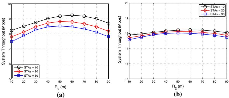
Fig. 5 Throughput performance of the DRP-PC scheme with various  $R_2$  values: (a) for short data-packet transmissions; (b) for long data-packet transmissions
