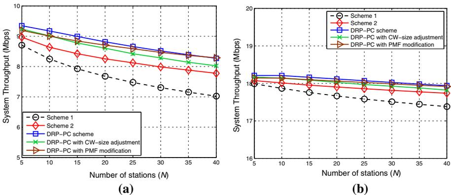
**Fig. 7** Comparison of system throughputs among different schemes ( $R_2=50$  m): (a) for short data-packet transmissions; (b) for long data-packet transmissions
