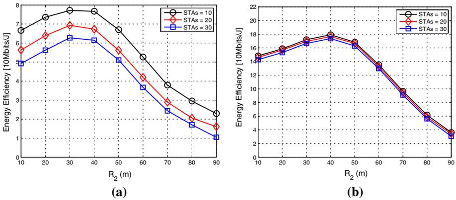
**Fig. 6** Energy efficiency of the DRP-PC scheme with various  $R_2$  values: (a) for short data-packet transmissions; (b) for long data-packet transmissions
