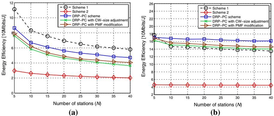
**Fig. 9** Comparison of energy efficiency among different schemes ( $R_2=50$  m): (a) for short data-packet transmissions; (b) for long data-packet transmissions.
