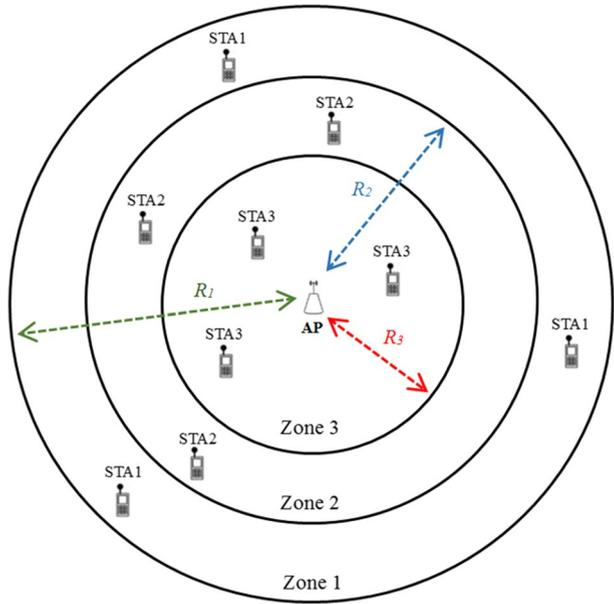
period, the transmission-power levels of the STA<sub>j</sub>s in Zone *j* are adjusted to have the same reception-power level, denoted as  $P_{rj}$ . Thus, there are *K* distinct reception-power levels, with each level corresponding to one of the *K* zones. Moreover, it is requested that  $P_{ri} < P_{rj}$ , if  $1 \leq i < j \leq K$ .
