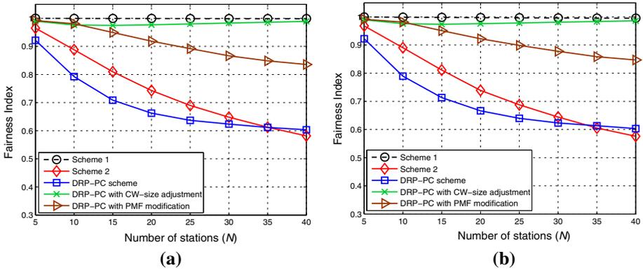
**Fig. 8** Comparison of the fairness index among different schemes ( $R_2=50$  m): (a) for short data-packet transmissions; (b) for long data-packet transmissions
